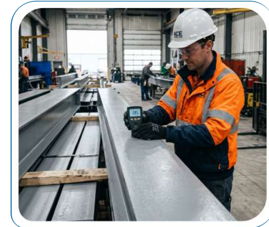
DFT Paint Verification
